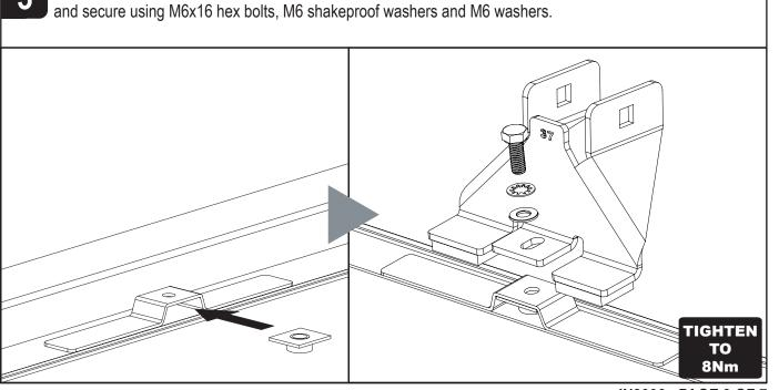
Secure roof brackets to the vehicles fixing points by placing the roof bracket plates under the fixing points
