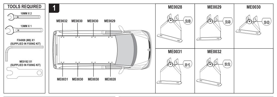
2 Stick rubber pads to the underside of the roof brackets. If fitting to an extra long wheelbase van (L3), place the small rubber pads (MA6019) in the front position on the rear brackets (ME0031 & ME0032) to level the bracket.
