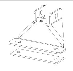
**3** Vehicles with threaded insert fixing points: Secure roof brackets using M6x16/25\* hex bolts (\*check fixing points thread depth), M6 washers and rubber washers. (FIG.1)
