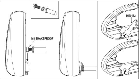
Assemble the roller spigot, M8x20 hex bolt and M8 shakeproof washer together. Place the assembly into the roller. Slide the roller onto the spigot fitted in step 12 and drop the other end into position. Tighten using the supplied tool (ME0182).
