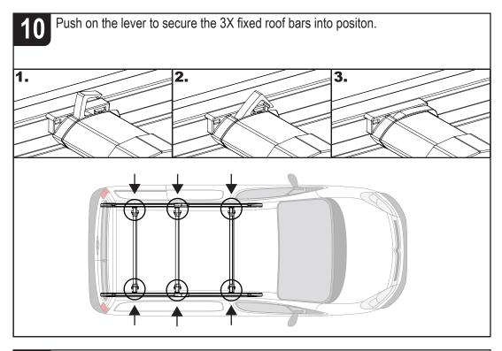
Place the remaining roof bars into position. See page 2 for the recommended distances between the roof bars. Once in position push on the lever to secure in place.
