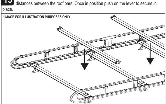
Place the remaining roof bars into position. See page 2 for the recommended
