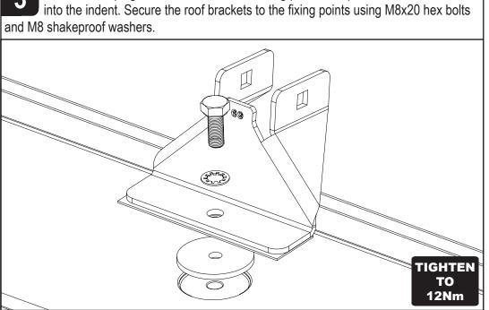
Remove roof plugs to reveal the vehicles fixing points and place rubber washers
