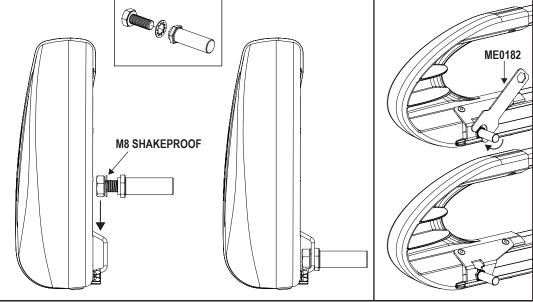
Assemble the roller spigot, M8x20 hex bolt and M8 shakeproof washer together. Place the assembly into the roller. Slide the roller onto the spigot fitted in step 14 and drop the other end into position. Tighten using the supplied tool (ME0182).
