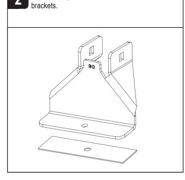
Stick rubber pads to the underside of the roof
