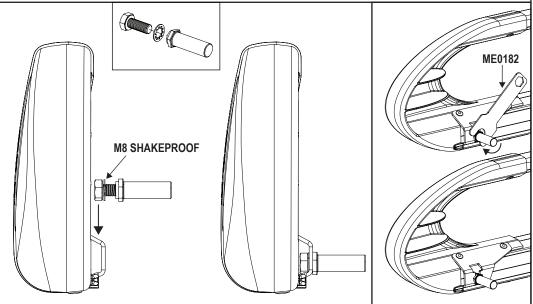
Assemble the roller spigot, M8x20 hex bolt and M8 shakeproof washer together. Place the assembly into the roller. Slide the roller onto the spigot fitted in step 11 and drop the other end into position. Tighten using the supplied tool (ME0182).
