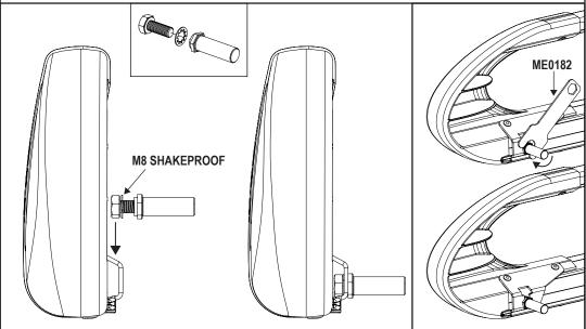
Assemble the roller spigot, M8x20 hex bolt and M8 shakeproof washer together. Place the assembly into the roller. Slide the roller onto the spigot fitted in step 13 and drop the other end into position. Tighten using the supplied tool (ME0182).
