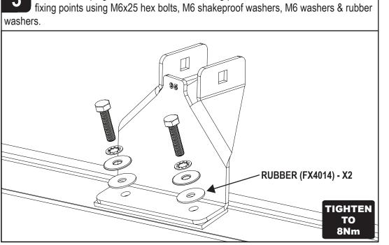
Remove roof plugs to reveal the vehicles fixing points. Secure roof brackets to the
