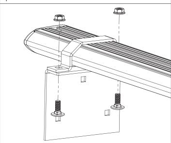
Slide the plastic covers on the van roof open to expose the roof fixing rail. If the van roof doesn't have plastic covers use the existing roof rail to clamp the roof brackets to.
