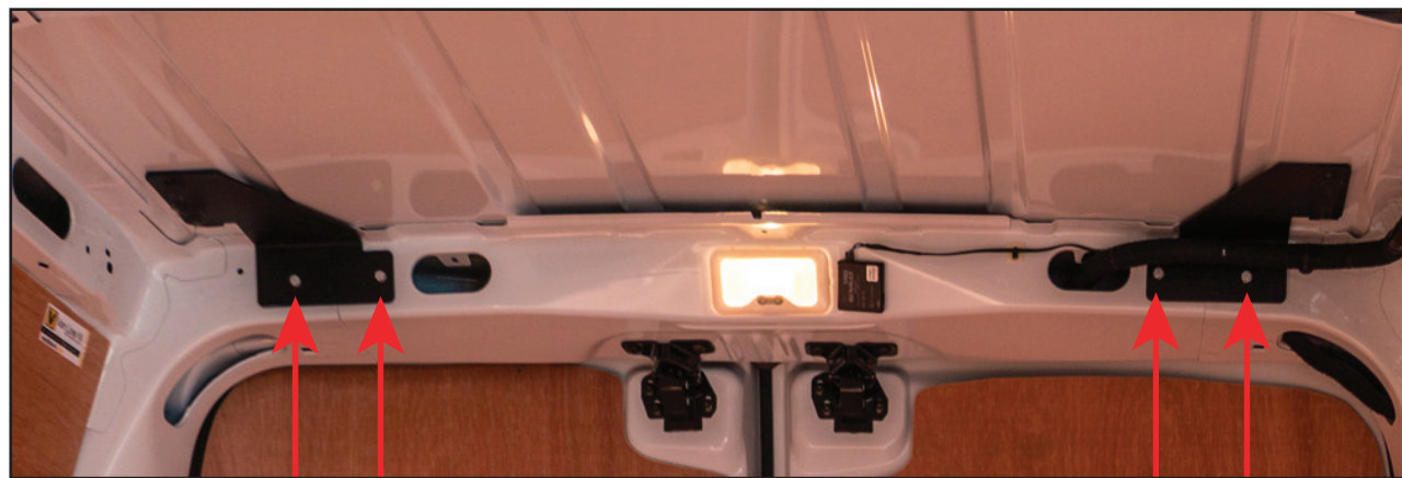
M6 1/4 TURN NUT INSERT LOCATIONS
